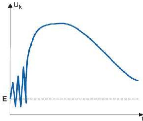
By coupling a capacitor  $C$  over the contact (see figure 3a) the voltage across the contact will be reduced and the voltage increase  $dU/dt$  will be limited to  $I/C$  instead of  $I/C_1$ .
