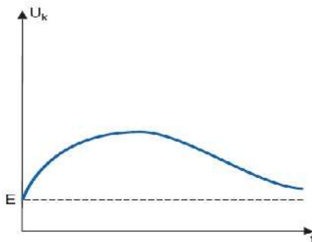
In order to limit the current through the contact when it closes, the resistor  $R$  must be connected in series with the capacitor. The values of the capacitor and the
