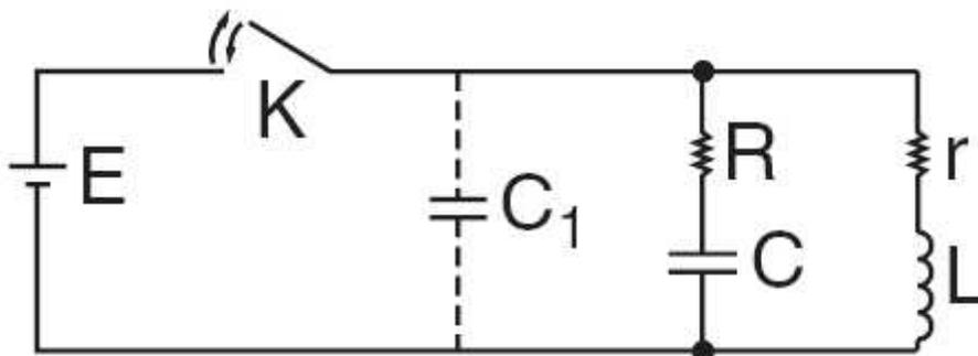
As  $I/C$  is much less than  $I/C_1$  the voltage increase over the contact will be kept low enough to prevent breakdowns (see figure 3b).
